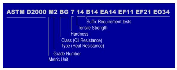
Specifications for physical properties of elasomeric seals can be very general or extremely specific in nature. Probably the most common general classification system is ASTM D 2000 Standard Classification System for Rubber Products in Automotive Applications. The purpose of this classification system is to aid in the selection of practical rubber products for specific environments. It also provides a line call out designation for the specification of materials.
